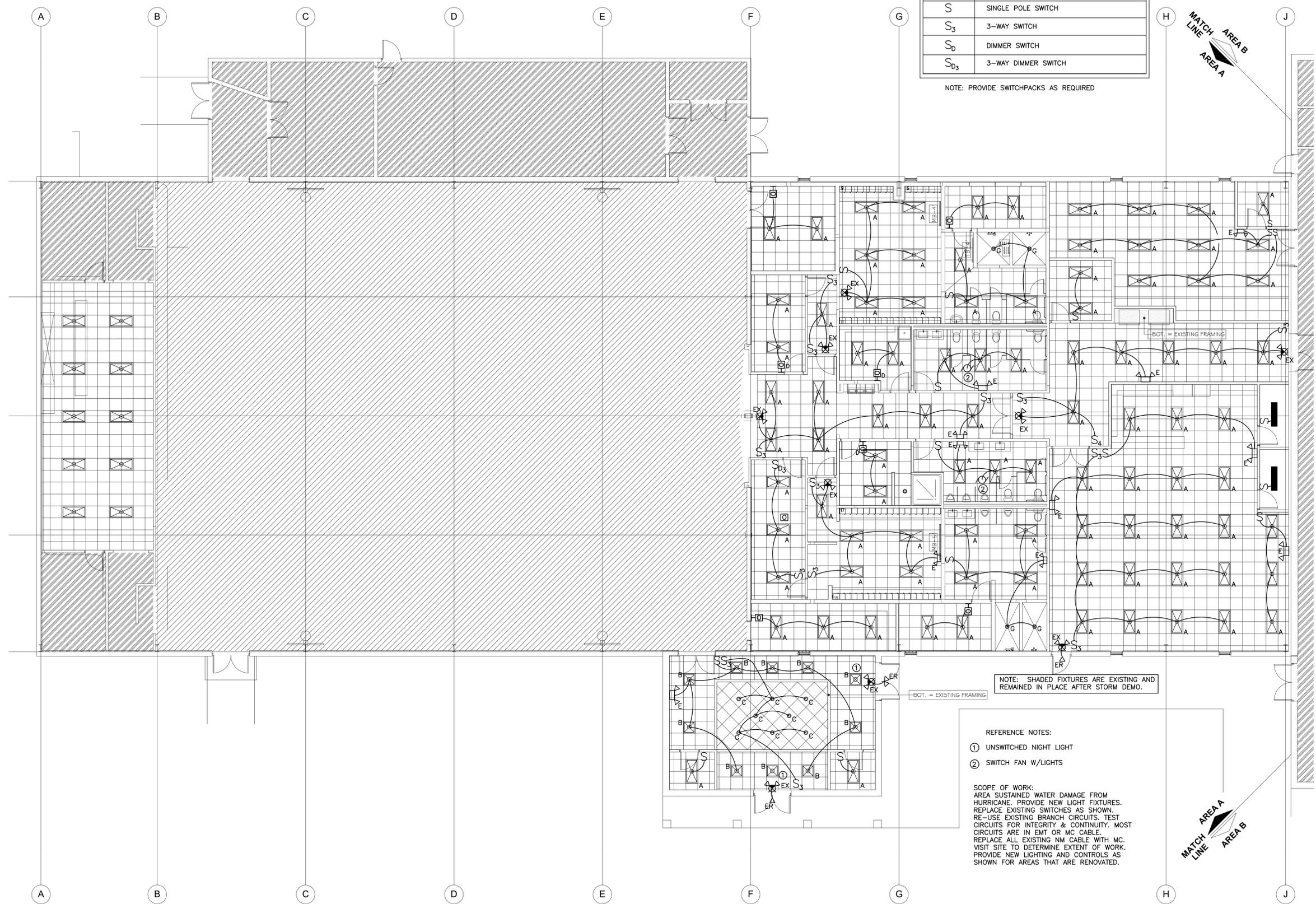
NOTE: SHADED FIXTURES ARE EXISTING AND REMAINED IN PLACE AFTER STORM DEMO.
