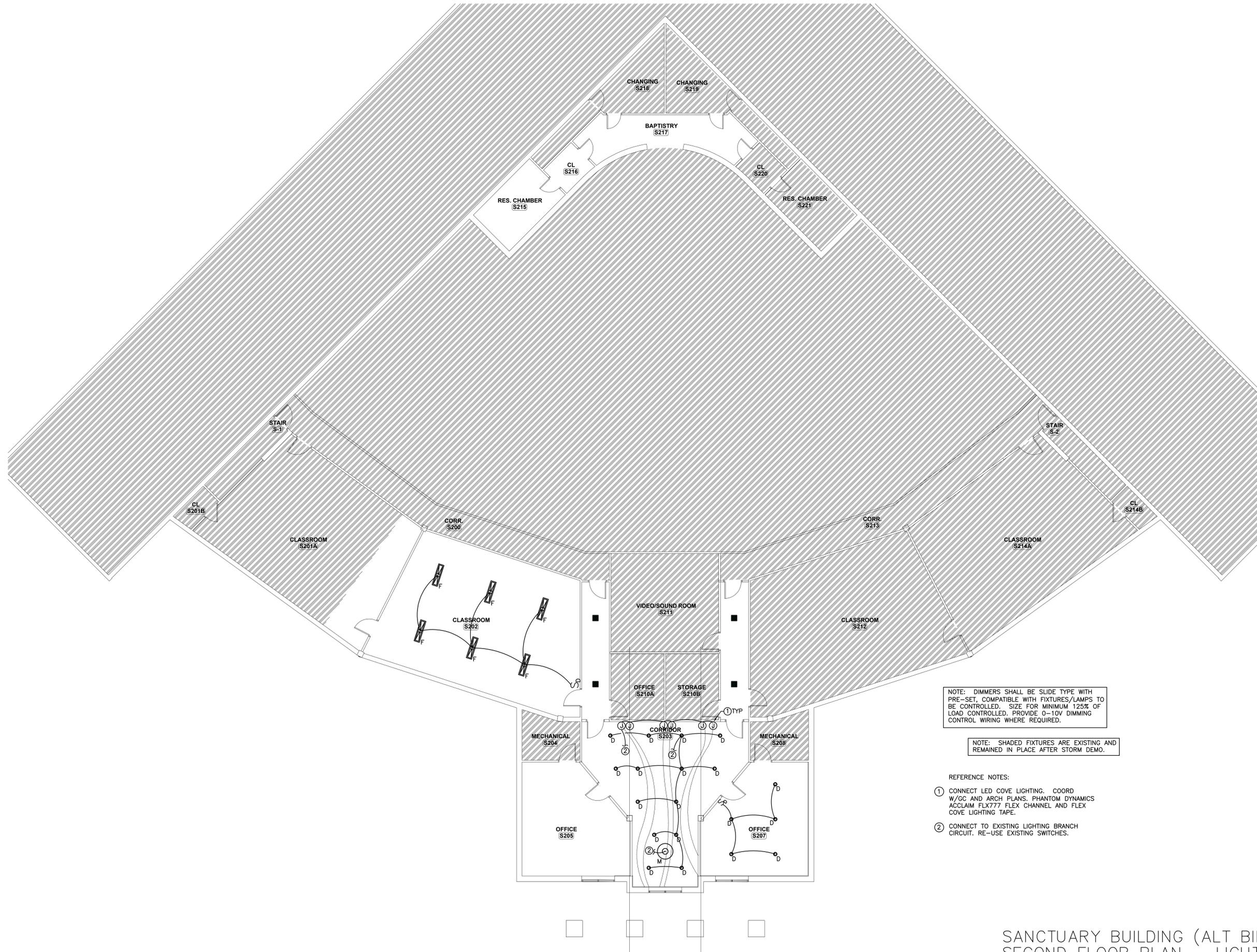
NOTE: DIMMERS SHALL BE SLIDE TYPE WITH PRE-SET, COMPATIBLE WITH FIXTURES/LAMPS TO BE CONTROLLED. SIZE FOR MINIMUM 125% OF LOAD CONTROLLED. PROVIDE 0-10V DIMMING CONTROL WIRING WHERE REQUIRED.
